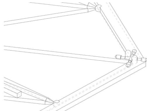
*Figure 5.2.1: Perpendicular (pitch/roll) hydrazine thrusters* *Figure 5.2.2: Planar (yaw) hydrazine thrusters*
