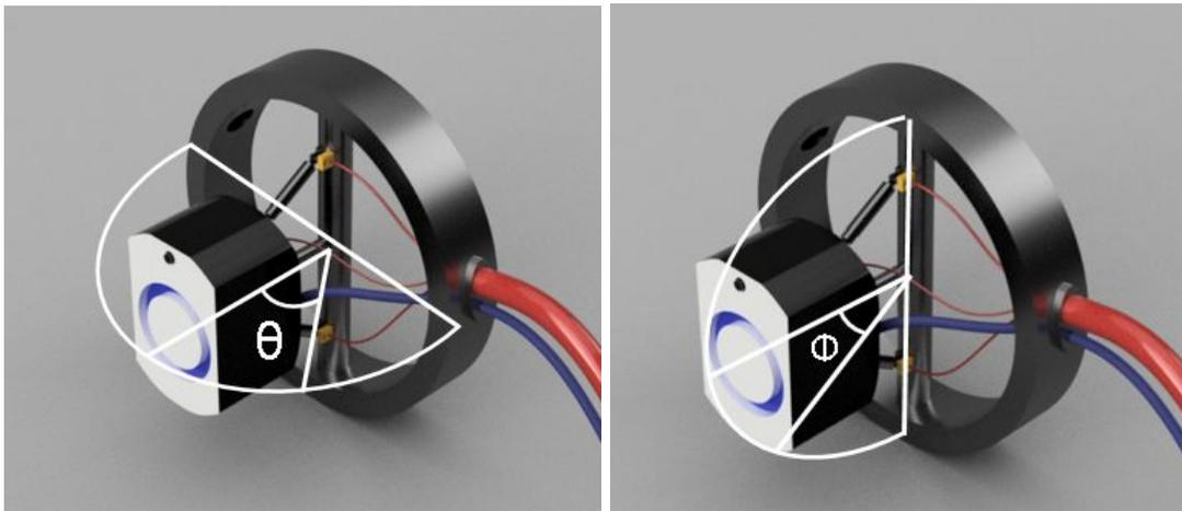
*Figure 4.3.1: Engine lateral swivel*
