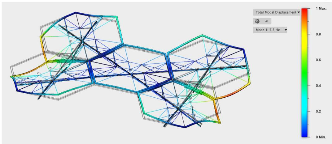
*Figure 6.1.1: Vibrational analysis of module truss system*
