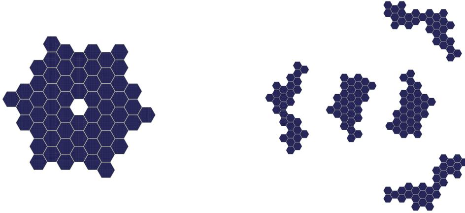
*Figure 5.7.1: Standard Sunflower configuration options, 12-module 291 kW configuration (left) and 30-module 727 kW (Right).*
