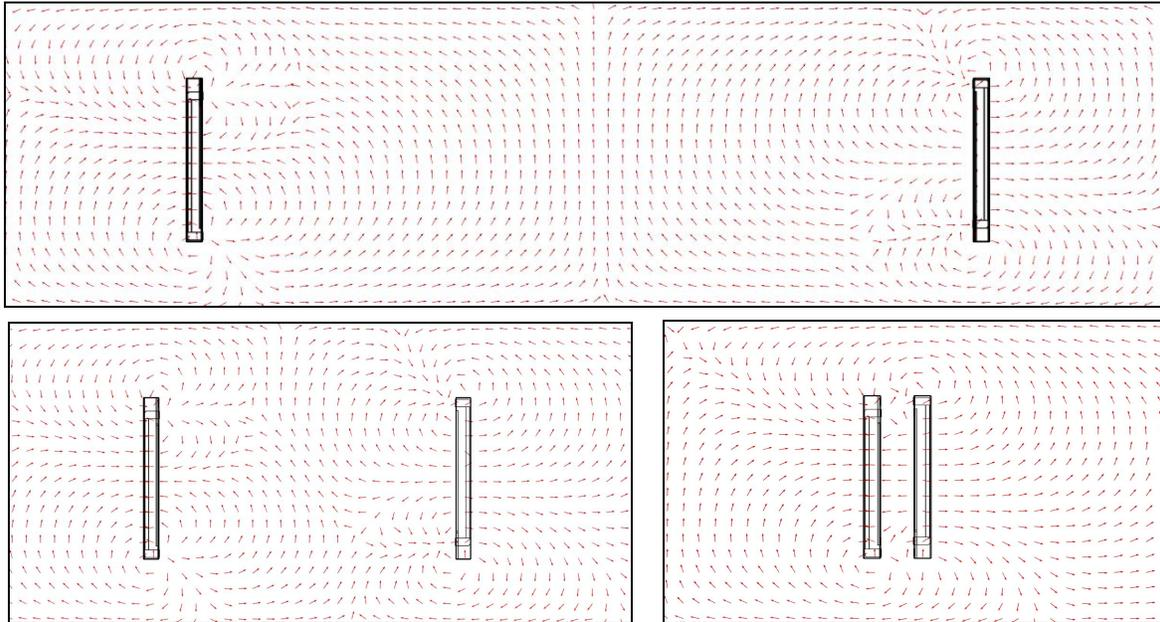
*Figure 6.4.1: Normalized magnetic field lines in two-joint system, with joints spaced 5 m (top), 2 m (bottom left), and 0.2 m (bottom right) apart.*
