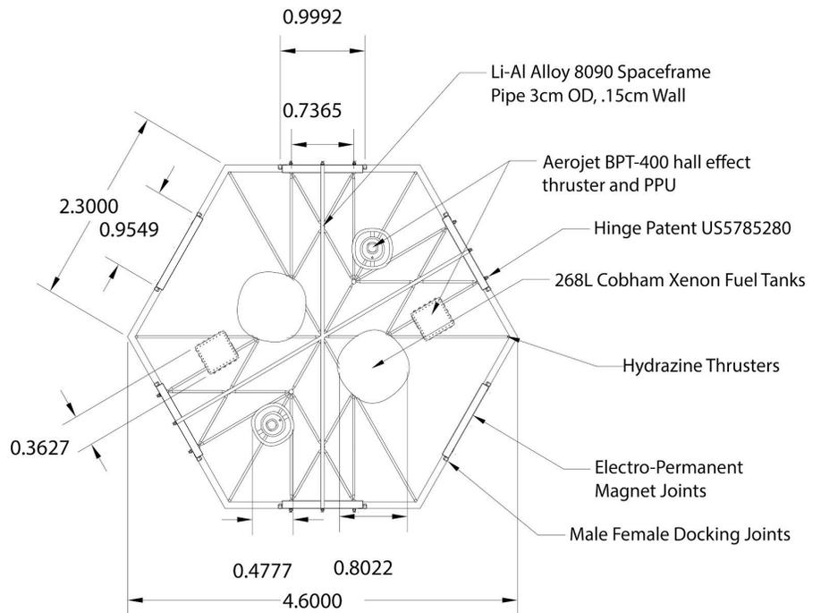
Figure 2.0.4: Schematic of central panel
