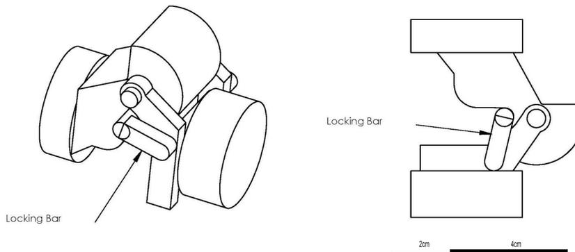
*Figure 4.2.1: Hinge joint connecting hexagons and allowing modules to unfold*
