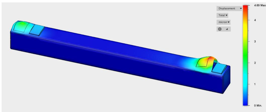
*Figure 6.2.1: Magnet Joint Displacement Under 8900N Load*
