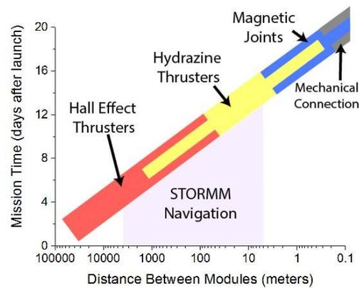
*Figure 5.0.1: Module aggregation timeline, starting at the release of modules from launch vehicle cargo fairing in LEO, and ending with magnetic and mechanical docking connection engagement.*
