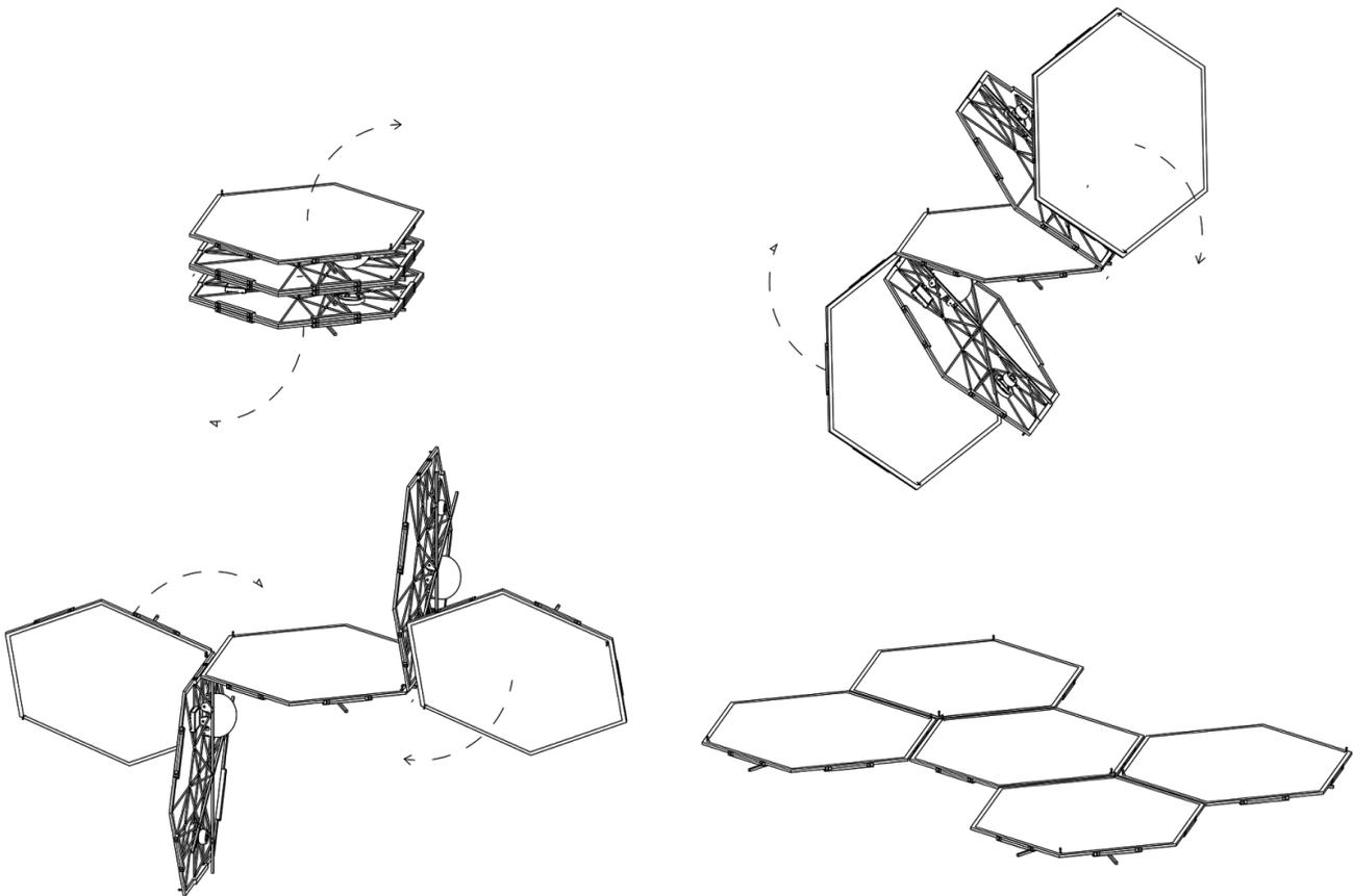
*Figure 3.2.1: Single Module Folding Sequence*
