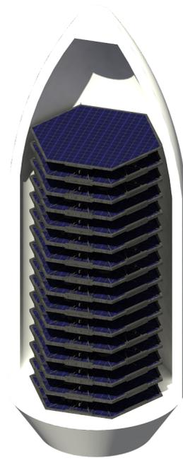
*Figure 3.1.2: Payload launch configuration*
