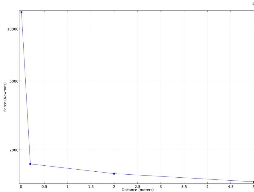
*Figure 6.4.2: Magnetic force between two electropermanent joints as a function of spacing between joints.*
