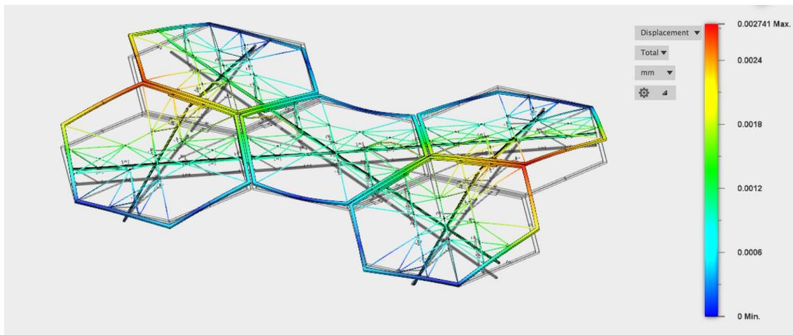
*Figure 6.2.2: Deflection analysis under 0.4 g acceleration of support frame from the thrusters*
