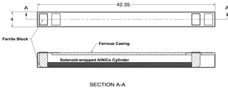
Figure 5.3.1: Schematic drawings of Magnet Joint
