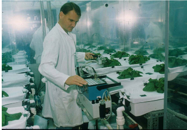
Figure 17.11: Neil Yorio at NASA's Kennedy Space Center taking leaf porometer measurements with potatoes to monitor stomatal conductance and transpiration rates. When measurements were taken at 400 ppm CO 2 , a mask was worn to removed exhaled breath from the chamber to avoid elevating the CO 2 concentration.
