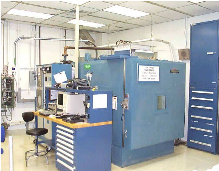
Fig. 2. Thermotron – set up for plant growth simulation under Martian conditions (KSC NASA).
