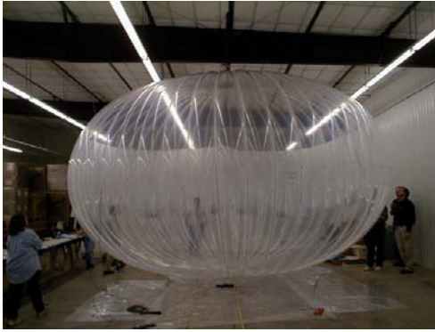
Figure 8 Ultra Long Duration Balloon (ULDB) super-pressure 'pumpkin' balloon prototype (Anon. 2000).
