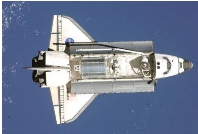
Figure 6. View of the Space Shuttle Orbiter Atlantis on approach to the International Space Station (ISS) during the STS-122 mission. Visible in the payload bay are the European Laboratory / Columbus module, the Integrated Cargo Carrier-Lite, the Orbiter Boom Sensor System, and the Shuttle Remote Manipulator System. Photo credit: NASA.
