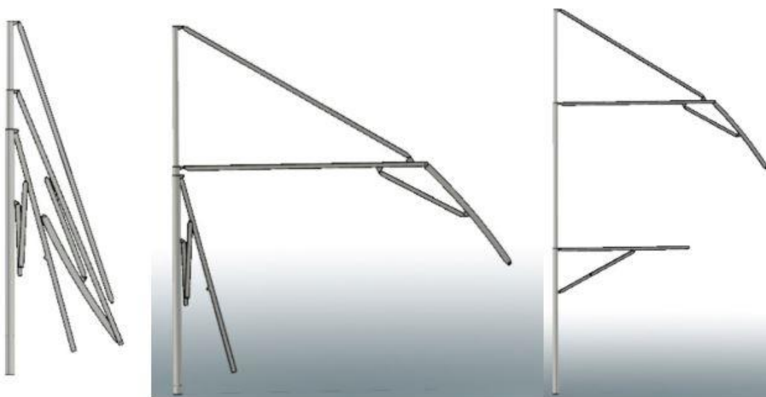
Figure 8: From left to right- represents the three stages in which the greenhouse will inflate.
