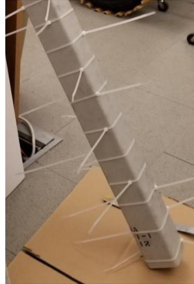
**Figure 7:** Distributed clamping of enclosed beam section.
