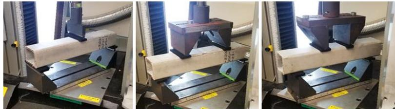
**Figure 25:** Flexural Testing of Teklam frame
