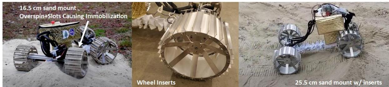
**Figure 21:** Snapshots of a SHREW operating in sand with and without wheel inserts.
