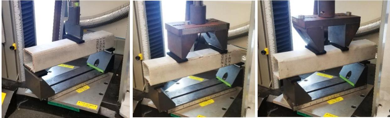
**Figure 9:** a.) 3-point setup b.) 4-point, quarter length c.) 4-point, third length.
