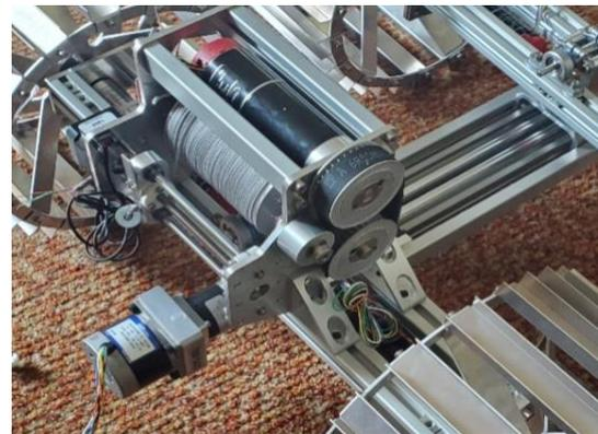
**Figure 13:** Winch mechanism for Earth prototype.
