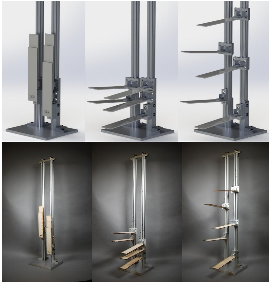
Figure 8: Deployment prototype in three configurations: packaged (left), partially deployed (center), and fully deployed (right). The top shows the CAD model, the bottom shows the physical version [40].
