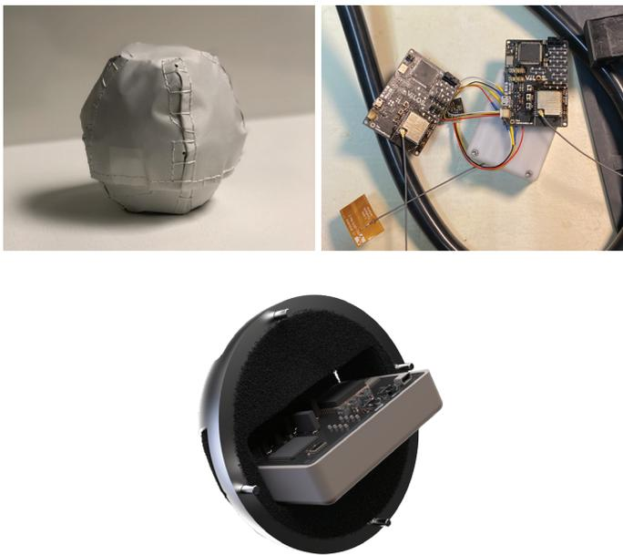
Figure 2: Fully assembled probe with MLI outer blanket (left), probe PCBs (right), probe sensor (lower)
