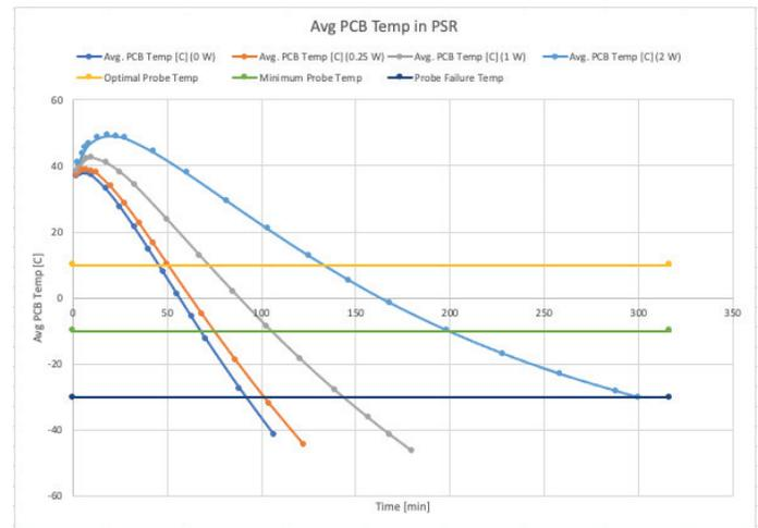
**Figure 21. Effect of Heater on Probe Lifespan**
