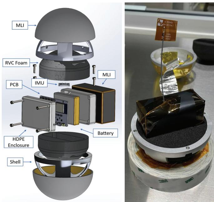
Figure 3: Probe CAD model exploded view (left), partially assembled probe (right)
