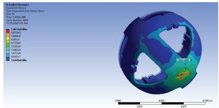
Figure 24. Stress Distribution in Shell at Peak of Impact
