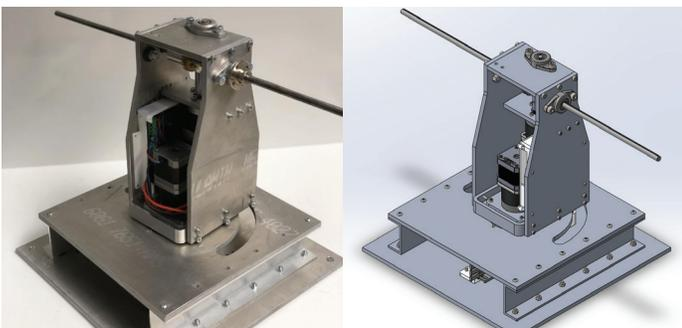
Figure 8. Launcher turret and base
