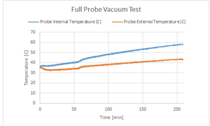
Figure 15. Temperature data from internal and external temperature sensors on the probe during vacuum test at ambient temperature
