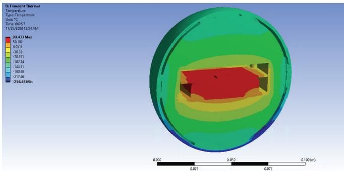
**Figure 20: Temperature Distribution of Probe Cross-Section After 3 Hours in PSR**
