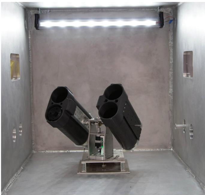
Figure 25. Launcher actuation in the azimuth axis
