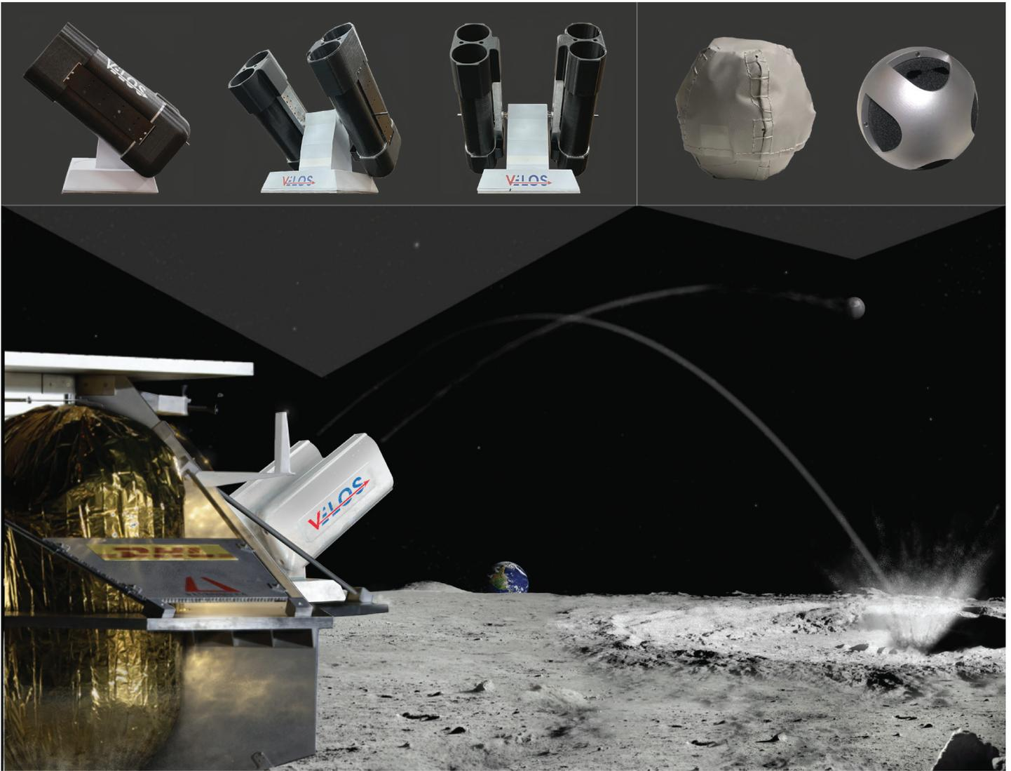
Figure 1: Graphic rendering of VELOS launcher on a CLPS lander
