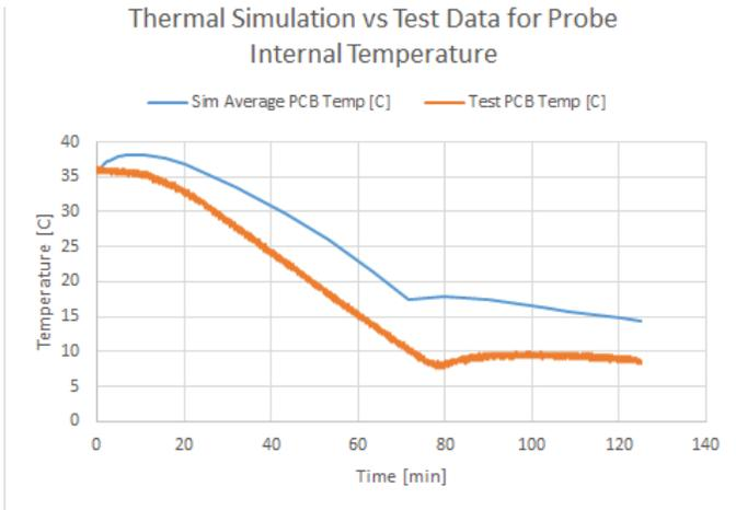
**Figure 19: Comparison of simulated and tested PCB temperatures**
