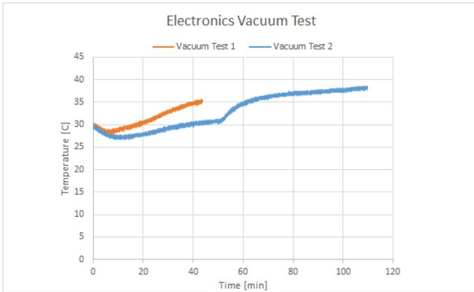
Figure 14. Temperature data from onboard sensor during vacuum tests at ambient temperature
