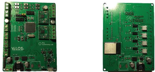
Figure 6. Top and bottom of populated launcher PCB
