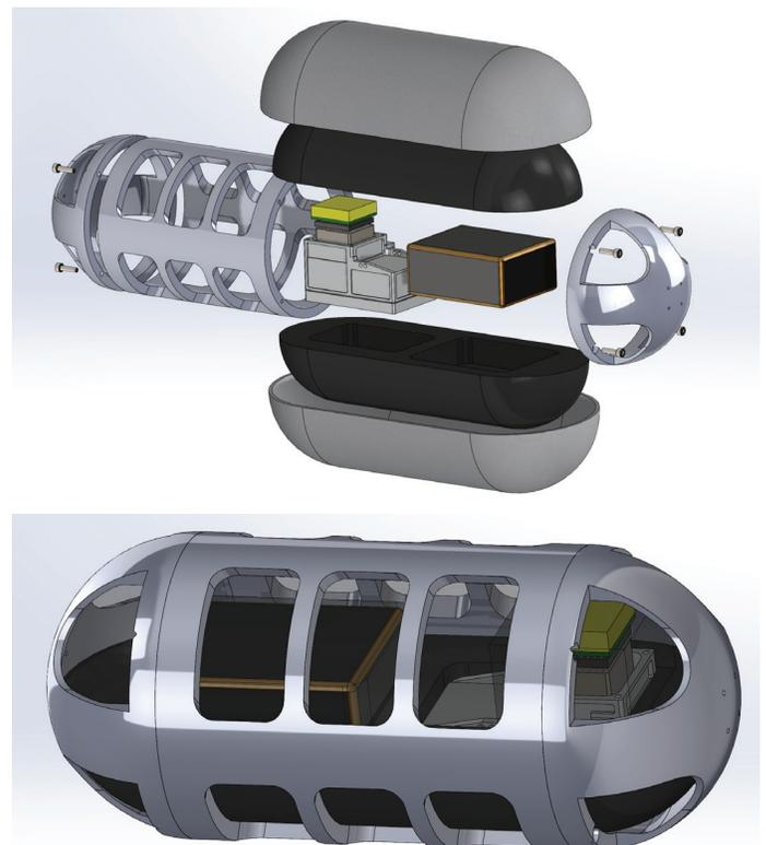
Figure 4. VELOS probe preliminary design to accommodate LunaH-Map Neutron Spectrometer
