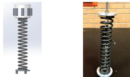
Figure 10. Spring and release mechanism subassembly outside of the barrel
