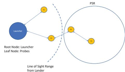
Figures 11. Mesh network diagram for Lander and Probes
