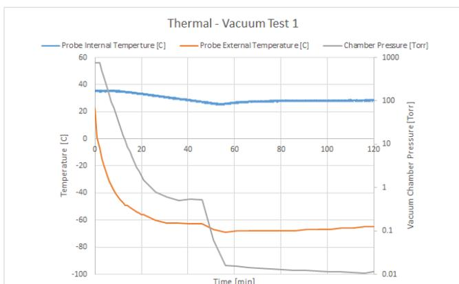
**Figure 17. Temperature data during in thermal-vacuum test #1**
