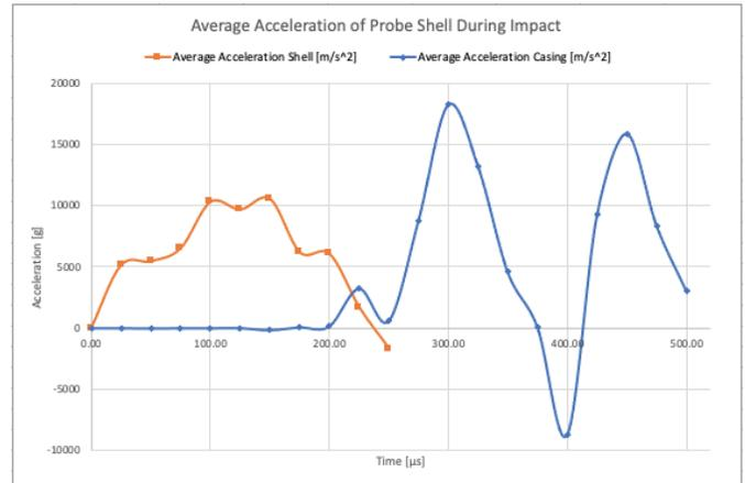
Figure 23. Shell and PCB Enclosure Acceleration Results
