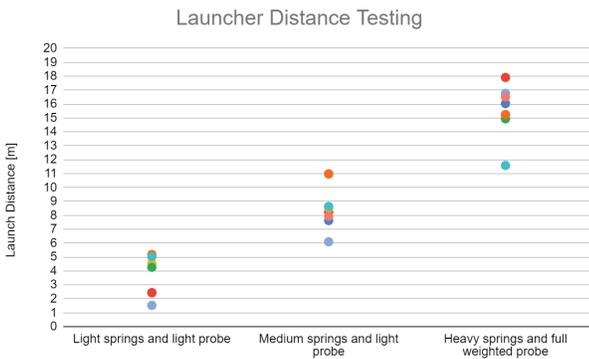
**Figure 27. Launch distance (from launcher to impact with ground plane) vs. test over the course of 8 weeks of testing**
