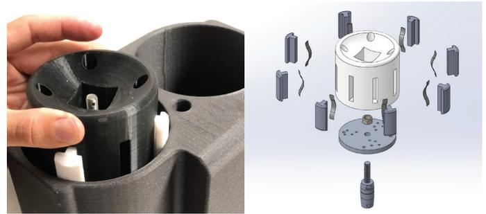
Figure 9. Plunger with PTFE (white) guides for smooth actuation and fit in the barrel
