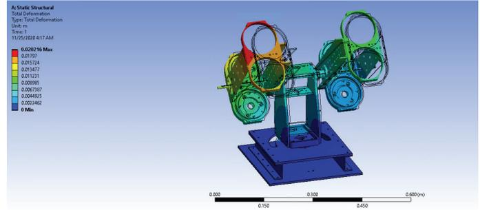
Figure 28: Deformation of Launcher Under Spring Load
