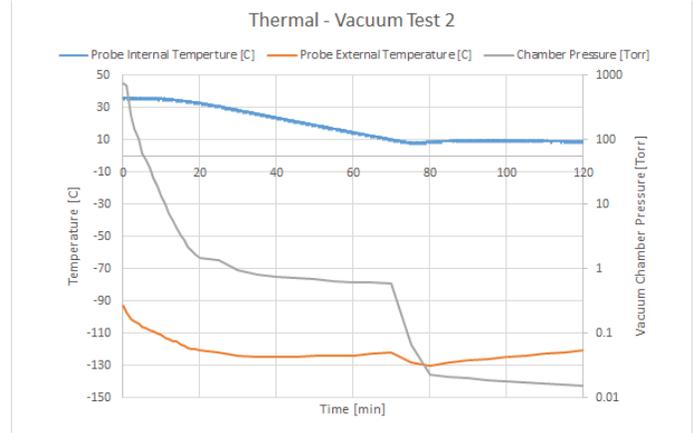
**Figure 18. Temperature data during in thermal-vacuum test**
