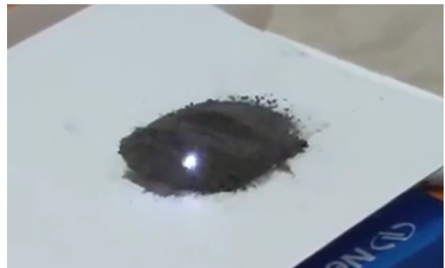
Fig. 14. The laser successfully ablates simulated lunar regolith.
