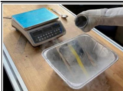
Figure 1 Using liquid nitrogen to remove lunar dust simulant with the Leidenfrost effect
