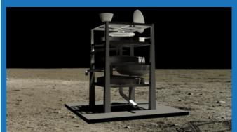
The Lunar Alloy Metal Production Plant or LAMPP is a self-contained, scalable, deployable metal production system designed for use in the lunar environment. LAMPP is based off the nascent technology of Molten Regolith Electrolysis which has been proposed as a possible way to extract metals on the lunar surface. The LAMPP system allows for a controlled MRE reaction, with oxygen as a byproduct, and the ability to extract pure metals or create metal alloys for further use.
