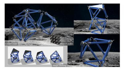
BYU proposes a modular, inflatable robot that can create a variety of different robotic structures on the moon. The robot consists of a set of inflated fabric tubes and robotic roller modules. The robot can change its shape robotically, and be structurally reconfigured based on the task at hand. The robot stows compactly, can lift heavy loads, and operate untethered. BYU will demonstrate this robot performing two tasks: a structure that can aim a solar array, and a crane that can lift loads.
