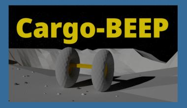
Cargo-BEEP is a two-wheeled inflatable vehicle, with the ability to autonomously navigate the lunar surface to assist astronauts in carrying cargo, either following astronauts during excursions or transporting supplies between locations. Cargo-BEEP is light and compact, expanding from a small cylinder. The vehicle would operate similarly to a Segway in principle and could be mounted on rovers or even on astronauts' suits while in compact form.
