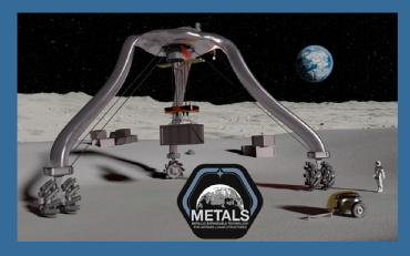
Metal Expandable Technology for Artemis Lunar Structures (METALS) is a versatile metal inflatable system that utilizes a novel combustive inflation process for inflation of efficiently packaged metal structures. METALS is designed to deploy from a compact storage configuration into a system of robust, expanded structures suitable for a variety of lunar applications such as gantries, towers, and other structural members.
