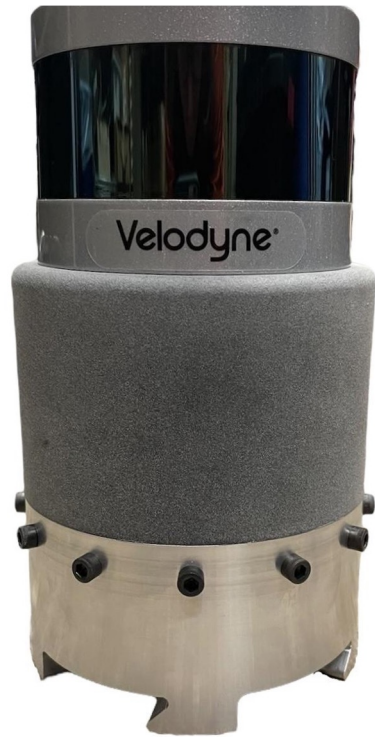
The “mapper” Species Module, with a LiDAR unit on top and a UIB Connector at the bottom.
