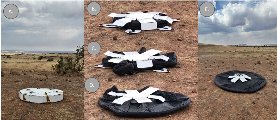
Figure 22. System Deployment: Anchor Actuation t = 0s (a.), Spring Release t = 34s (b.), Inflation begins t = 37s (c.), Partial inflation t = 55s (d.), Inflation Complete t = 76s (e.)
