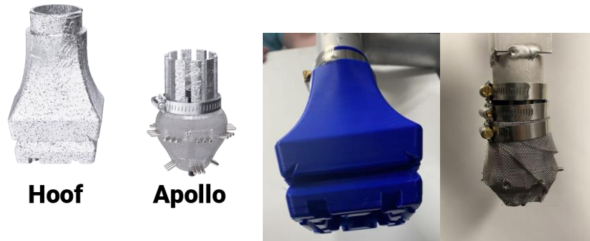
Figure 27. CHARLOTTE shoe prototypes, CAD renders (left), physical prototypes (right)
