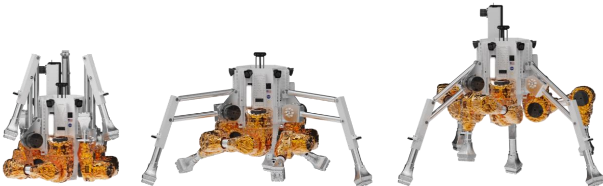
Figure 14: Fully stowed position for flight (left), Partial unfolded position (middle), Fully unfolded position (right)
