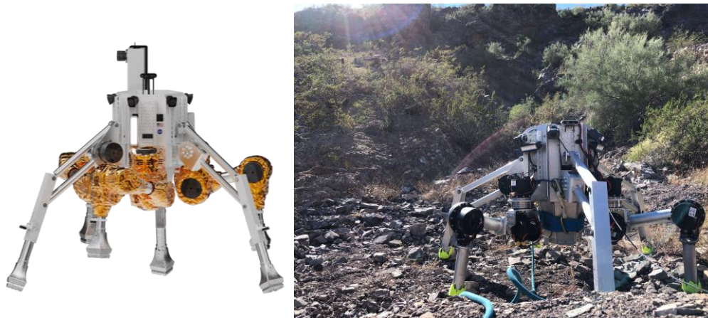
Figure 5: CHARLOTTE CAD model render (left), CHARLOTTE during Environmental Testing at Hayden Butte
