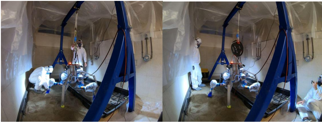
Figure 26. CHARLOTTE Dust Testing without gravity harness (left), with gravity harness (right)
