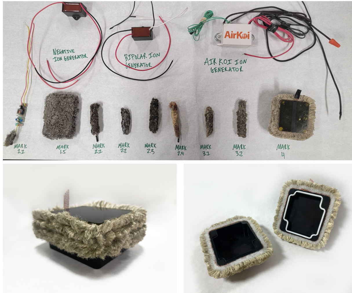
Figure 5. The evolution of TEST-RAD. Top row: All Marks of TEST-RAD lined up along with the bipolar generator iterations. Bottom row: The final Mark of our system, applied to a junction box.
