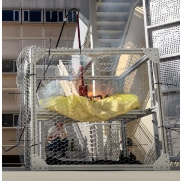
Figure 4-25: Hot fire test stand using 500,000 BTU/hr propane torch suspended over a cement plate with through holes for model mounting. The stand is wrapped in chicken wire to prevent burning material from blowing away.
