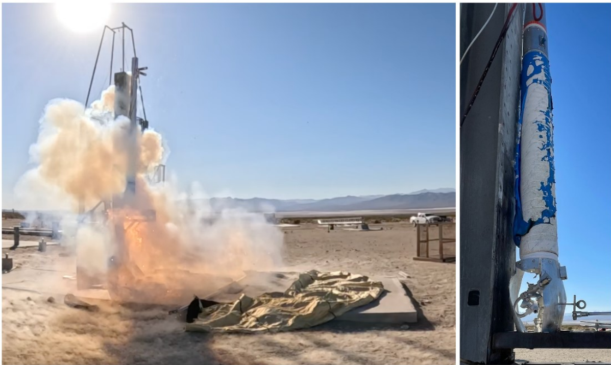
Figure 4-28: Photos from FAR test on October 21st, 2024. Pictured on the left is the PILLARS prototype anchored to metal struts secured on either side of the launch pad next to a failed rocket launch. On the right is the extensive damage done to the rocket motor by a valve failure in the LOX line.
