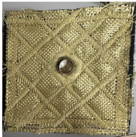
Figure 3-14: A nearly completed anchoring interface patch. Three layers are sewn together, with bi-directional cross-stitching. Dense stitching can be seen at the central connection hole acting as an edge finish. The bottom of the brass grommet has been placed in the center hole, and only the top of the grommet needs to be connected for a finished anchoring interface patch.
