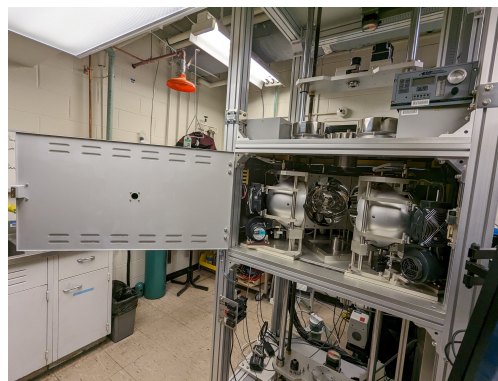
Figure 7: An image of the floating zone furnace set up for the un-beneficiated small-scale experiment
