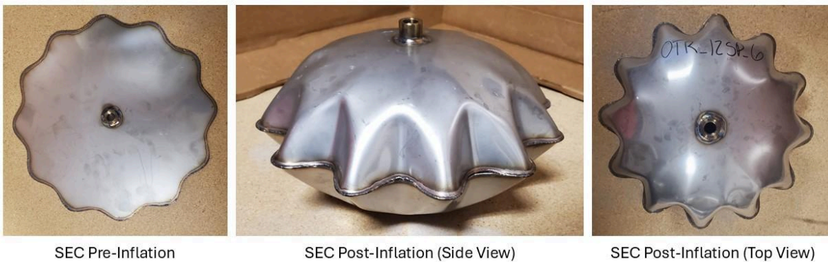
Figure 2: Images of optimized Sinusoidal-Edged Circle (SEC) design before and after deployment.
