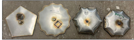
Figure 13: Repaired Modules with solid-state (1, 2) and liquid-state (3, 4) solutions.
