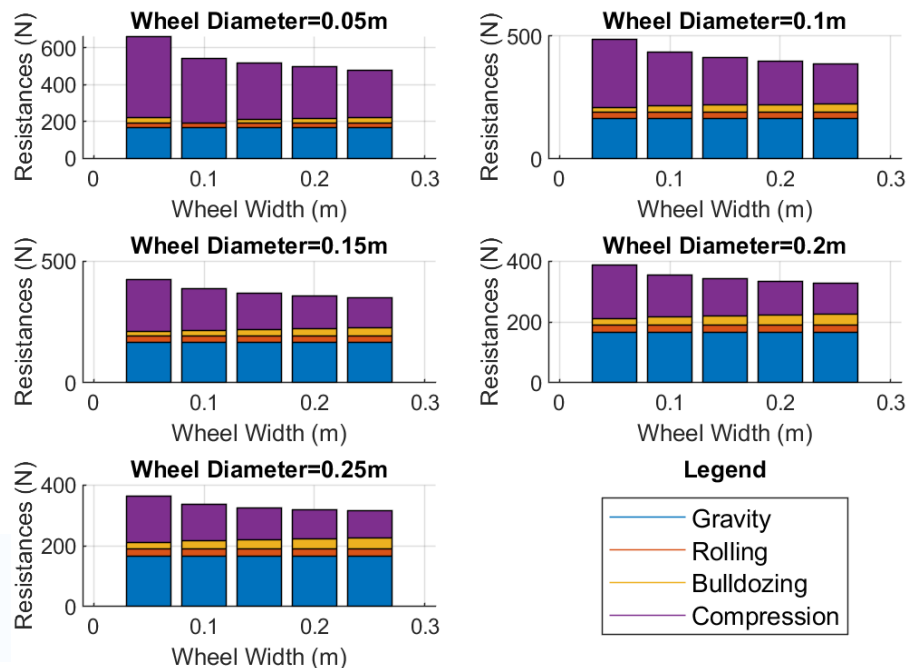
Resistances for 4 Wheels at Slope=20 deg, 300 kg
