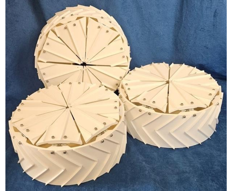
Independent triangular petals protect inflatable in stowed configuration and allow inflatable to conform to soil.
