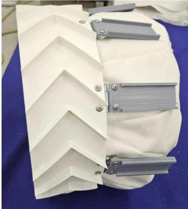
Early wheel design using existing wheel, retrofitted with deployable grousers and inflatable.
