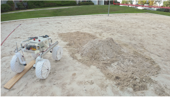
Fig. 22 Testing rover over slope with site seen
