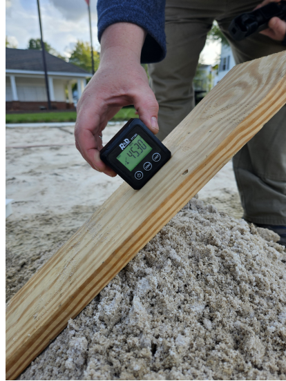
Fig. 23 Measured angle of the test slope using digital inclinometer
