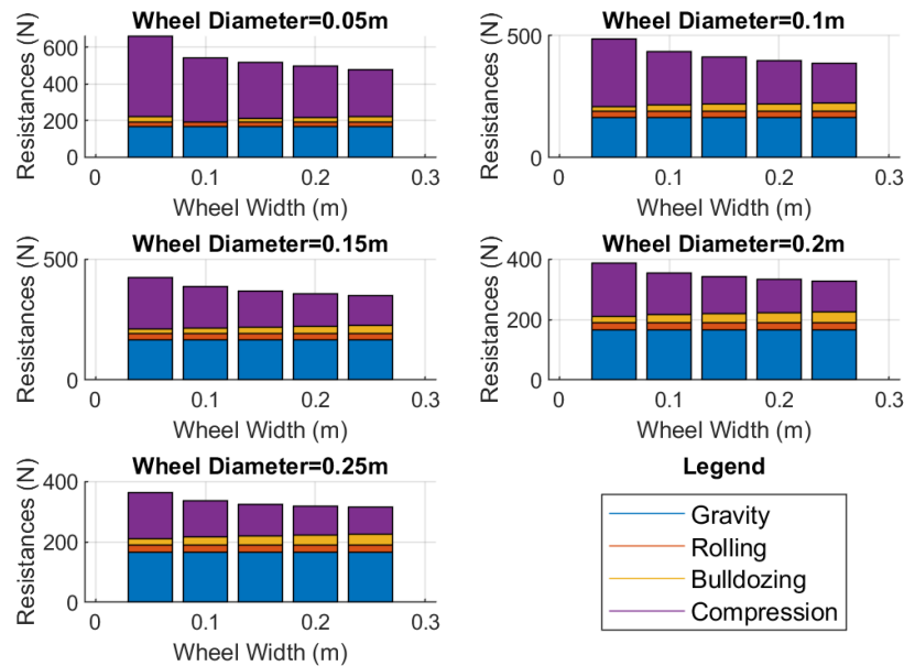
Fig. 2 Terramechanics soil resistances for a variety of wheel geometries, with wider wheels experiencing less overall.
