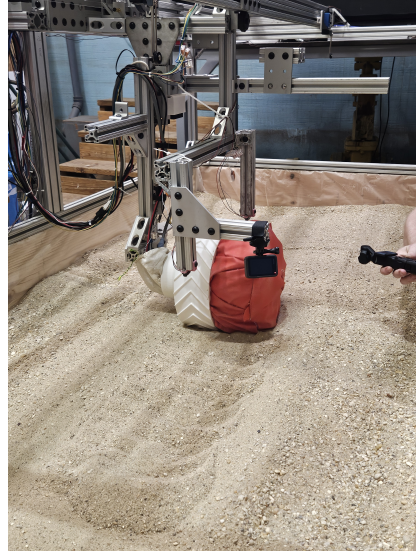
Fig. 8 Testing the performance of a deployed inflatable without grousers
