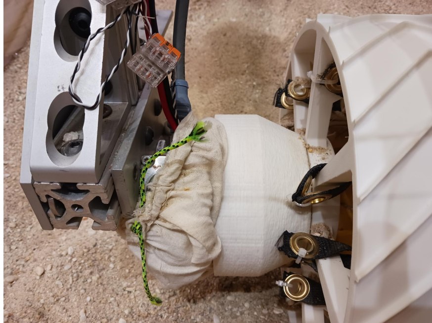
Fig. 15 The force/torque sensor now has an environmental protection garment, and the wheel drive motor has a 3D-printed cup to protect from sand and dust
