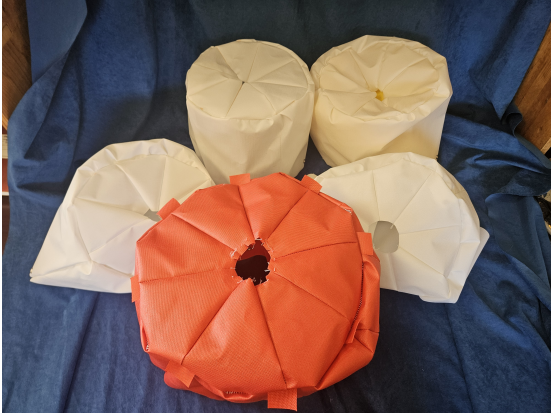
Fig. 7 A variety of the restraint layers produced and tested
