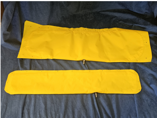
Fig. 9 The final two pressure bladder designs
