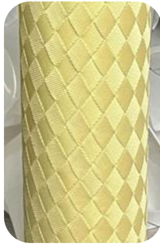
Figure 21: 90 degree helical pattern.
