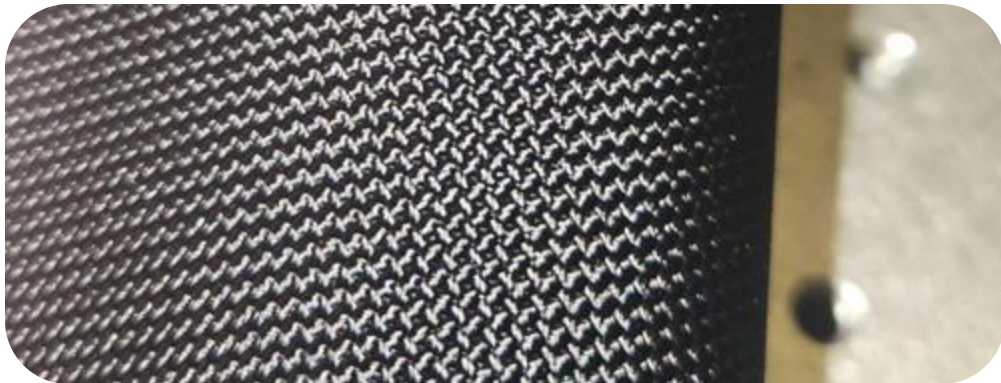
Figure 44: Ballistic Nylon is coated with Polyurethane, demonstrating the material's glossy aspect.
