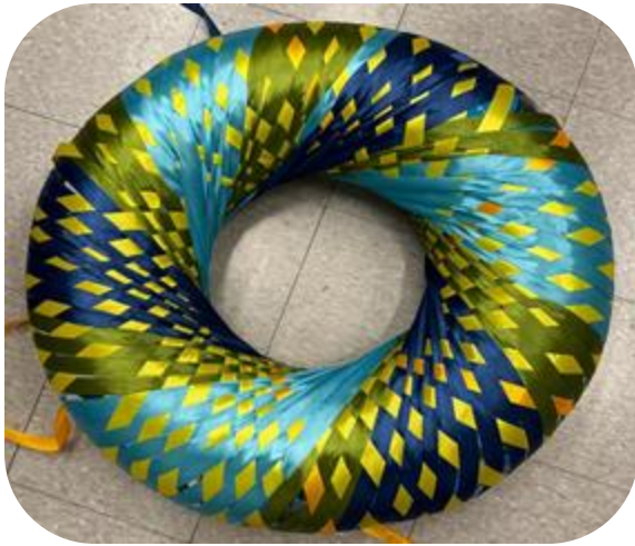
Figure 20: 45 degree torus weave pattern woven around commercial off the shelf (COTS) scaffold.
