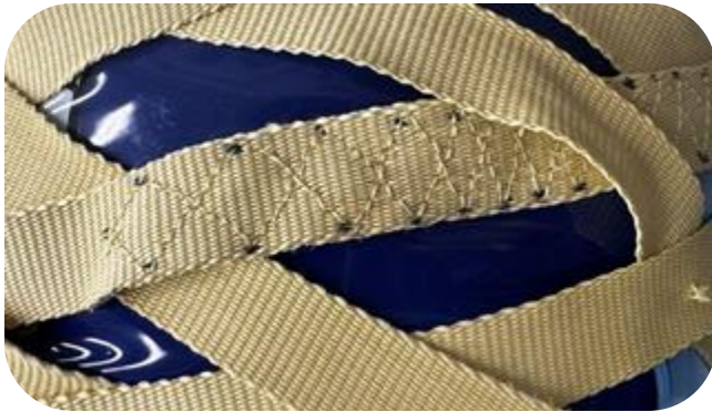
We used a tapered diamond stitch to attach new straps to the ends of other straps.
