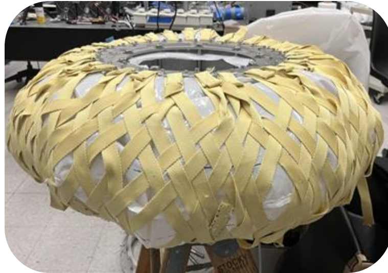
Figure 35: Inflated wheel with hermetic and restraint layers.
