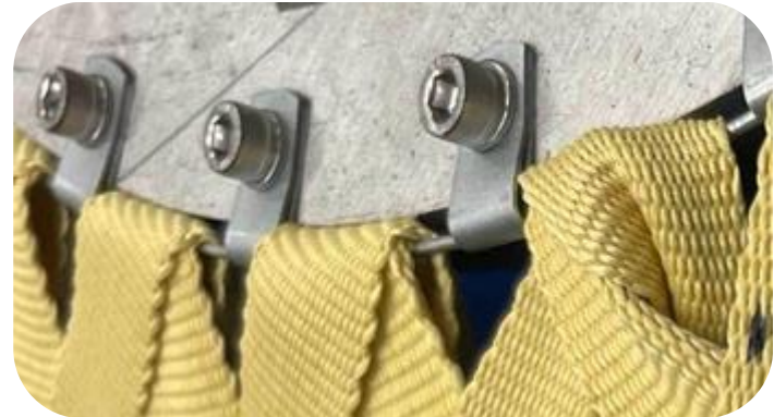
Figure 37: Clevis roller inspired strap connections for restraint layer.
