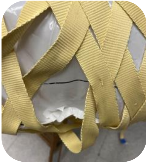
Figure 34: Patching on the hermetic layer
