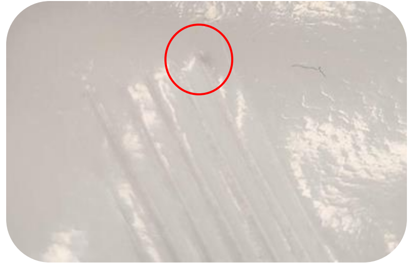
Figure 33: Metal brackets on the heat sealer created micro holes during sealing.
