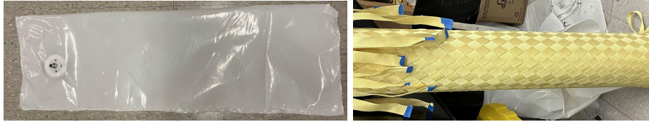
Figure 8. (Left) Hermetic layer. Shows the PTFE gasket seal and the PET plastic layer heat sealed around it. (Right) Restraint layer during fabrication. Note the cross-hatched “finger trap” design that will pull taut as the robot expands.
