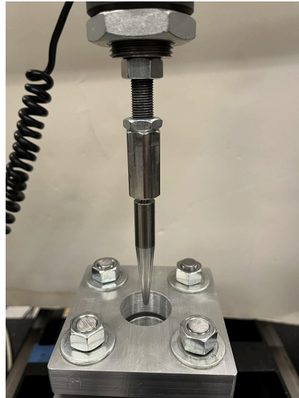
Figure 16. The ASTM F1306–21 puncture testing rig mounted in the Instron load frame.
