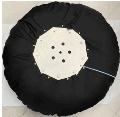
Figure 2. Wheel inflated with fill system and all layers.
